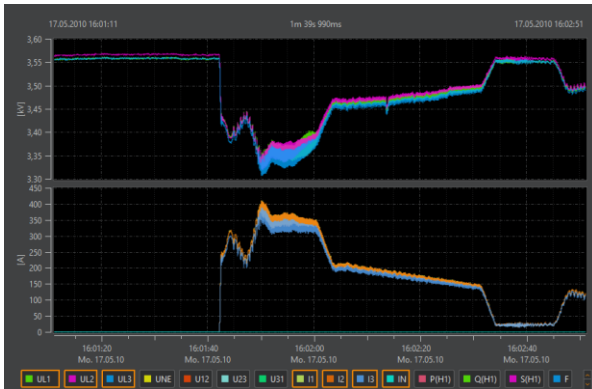
10 ms half cycle record (example machine start-up)
